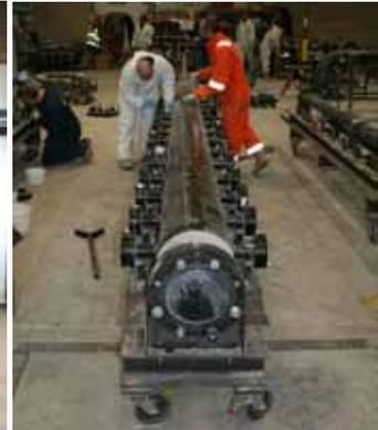
Headers assembled in the jig, with the branches bonded and ready to wheel into the oven.
