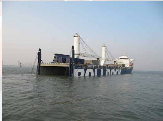
Rolldock's new heavy lift ships have three modes of loading and unloading – lolo, ro-ro and submerging
